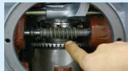
Internal gear check
